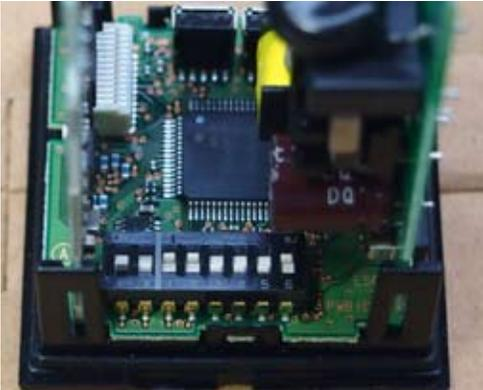
Use a small screw driver to set the dip switches on the controller as shown.
