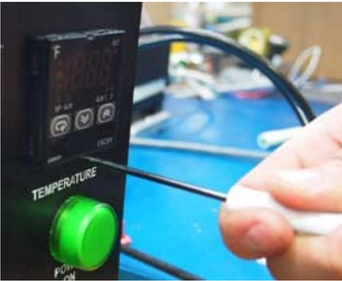
Use a small screw driver to release the latch holding the Controller in place.
