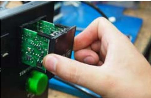
Pull the controller all the way out of the enclosure.
